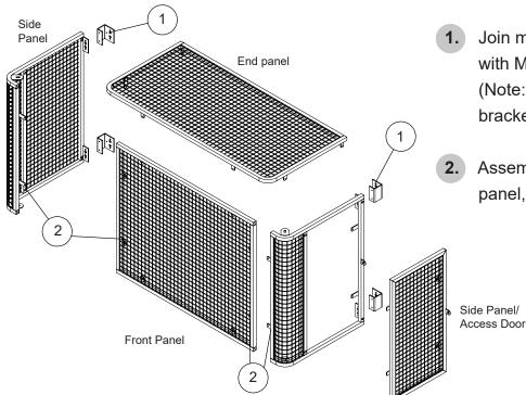
Join mounting brackets to side panel with M6 x12.
